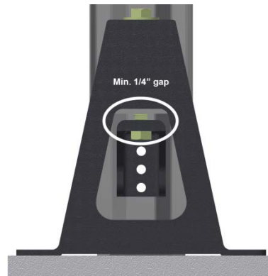
Figure 5: Leave 1/4" (+/- 1/8") gap between C-channel and bracket.
