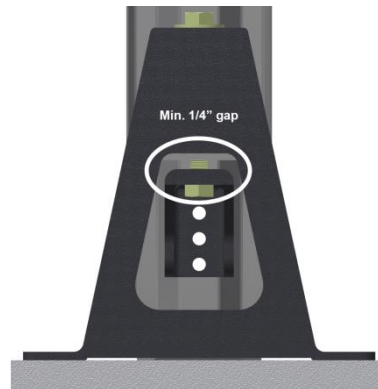
Figure 5: Leave \frac{1}{4} " (+/- \frac{1}{8} ") gap between C-channel and bracket.
