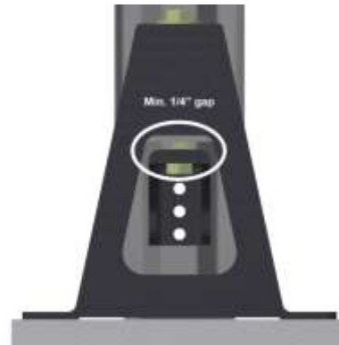
Figure 5: Leave 1/4" (+/- 1/8") gap between C-channel and bracket.
