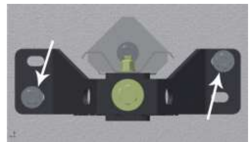
Figure 6: Drill anchor bolts 2 1/4" deep.
