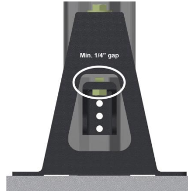
Figure 5: Leave 1/4" (+/- 1/8") gap between C-channel and bracket.
