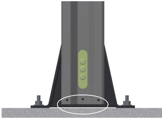
Figure 4: Lift until there is a 1/2" (+/- 1/8") gap.
